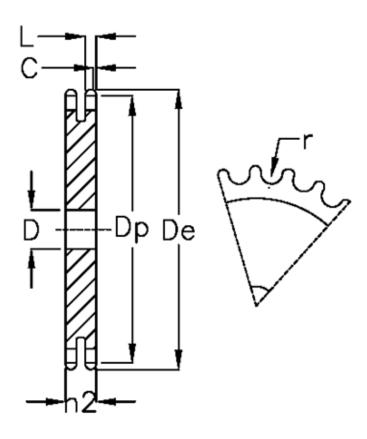
C = 2 D = 30 De = 563.9 Dp = 555.92 For chain size =  $5/8 \times 3/8$ For chain type = 10 B-2 h2 = 25.5
